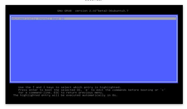
**Band OS** will install automatically. User input is not required. The installation process takes about five minutes.
